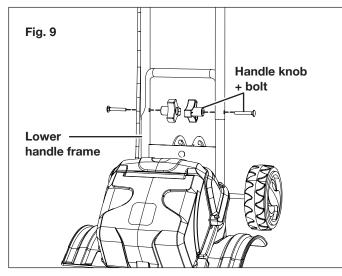
**NOTE:** Make sure that the handle knobs are placed inside the handle frame. Otherwise they will affect the wheel adjustment system.
