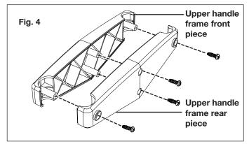
Fit the left upper handle and the right upper handle in the handle grooves of the upper handle frame rear piece. Make sure the holes are aligned (Fig. 5).
