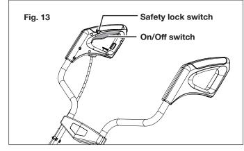
3. To switch OFF, release the ON/OFF switch (Fig. 13).
