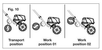
**2.** To adjust the wheel position, push the wheel adjustment knob while moving it to the slot for desired position; let go of the knob and make sure it locks into position (Fig. 11).
